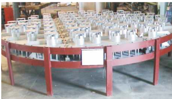
Check assembly of distributing trays on the reactor mock-up 3.6 m in diameter.
