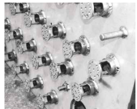
Distributors of gas-and-liquid sprays for superfine distribution (Patent #2281804)
