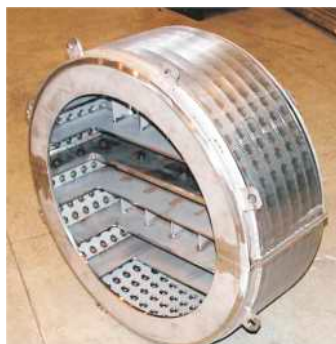
The bottom basket equipped with a wedge profile, which screen was produced by the Johnson Screens company
