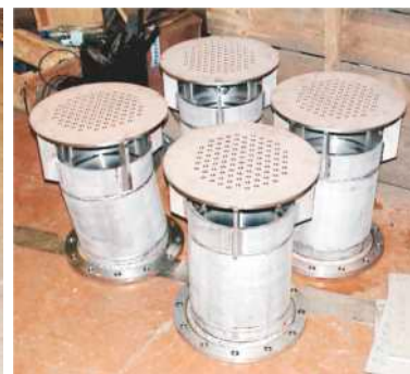
Upper distributor with perforated distributors
